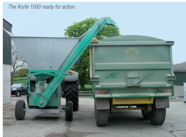
This tractor consumes just 18L/hr of red diesel to run the crimper.
